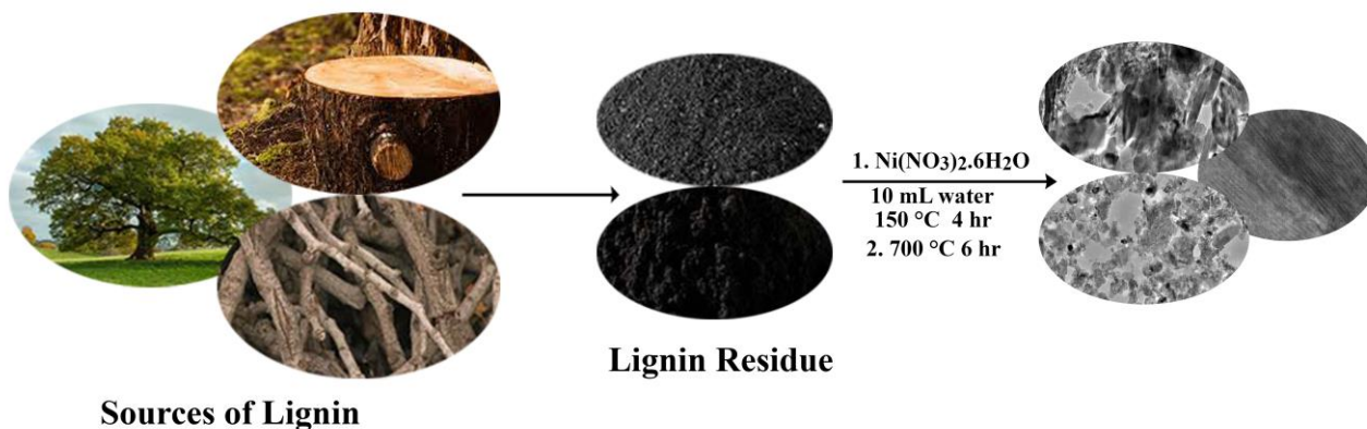
Scheme 1. Schematic illustration of the synthesis of NiO@LBM nickel nanoparticles.
